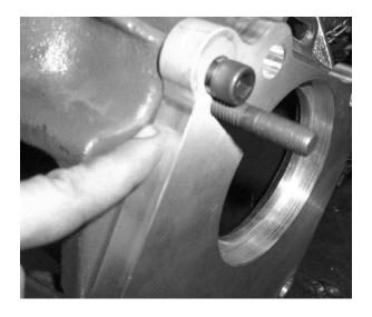
INSTALL THE TRANSMISSION TO ADAPTER PLATE BOLTS USING A THREAD LOCKING COMPOUND ONLY AFTER THE PLATE IS BOLTED INTO PLACE ON THE BELLHOUSING..
