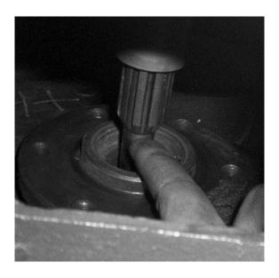
INSTALL THE FLYWHEEL, CLUTCH DISK AND PRESSURE PLATE. TORQUE DOWN THE ALL BOLTS IN A CRISS-CROSS PATTERN.
